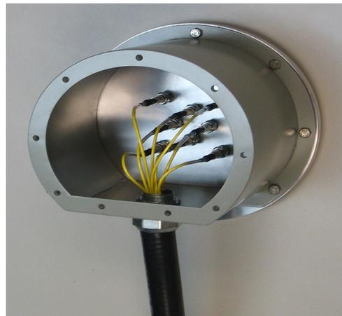
Fig. 7 Feedthrough fiber optic plate, with protection box
